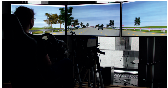
Figure 5: A simple driving simulator with eye tracker, e.g. for first tests on driver distraction.
