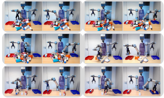
Fig. 6: Real robot performing the table cleaning task in three different levels of difficulties: highly cluttered, cluttered and isolated real-world scenarios.
