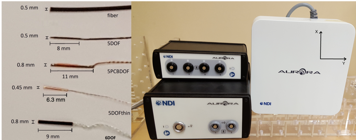
FIGURE 3.1 – Optical fiber, four EM sensors with their collecting cables (left panel) and Aurora V3 electromagnetic tracking system (right panel). These sensors were added to our scintillating fiber dosimeter. Axes are indicated on the field generator, with the Z axis coming out of the figure.
