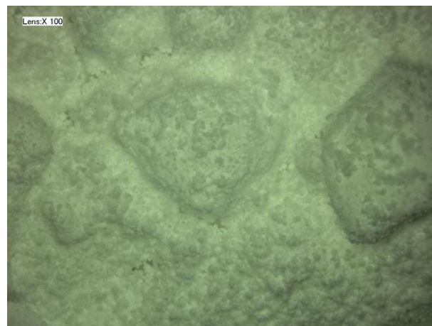
Figure 7. Digital microscopy picture of bound powder of a mixture of powders from experiments S14 and S15 (magnification x100).
