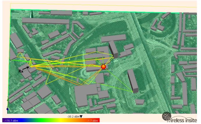
Fig. 10. Propagation paths between the Tx at 15m height and an Rx position
