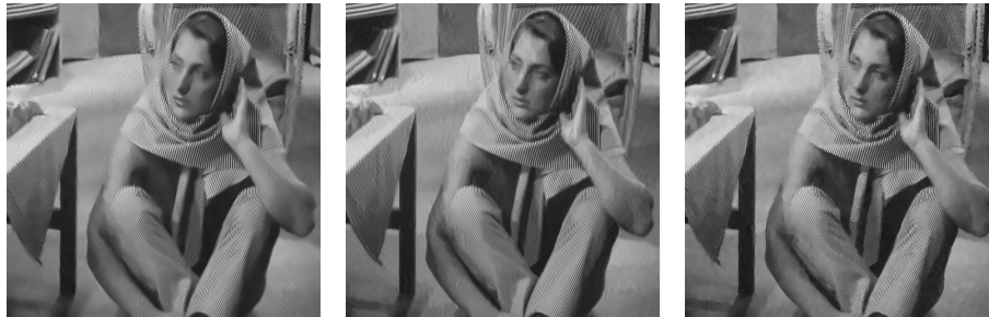
(c) NLMS restoration (28,86 dB) (d) BM3D restoration (29,57 dB) (e) Proposed NLMS-SC restoration (29,79 dB)
