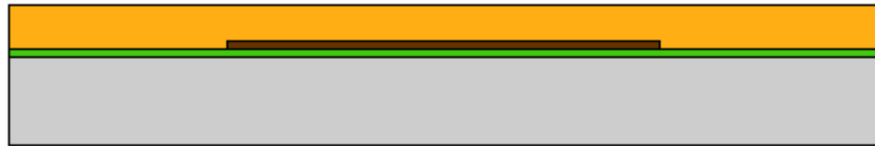
(a) Applying a polyimide and SU-8 layer
