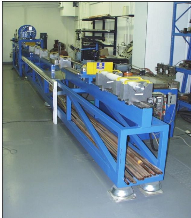
Figure 2: Split Hopkinson tensile bar setup at Ghent University. Its total length is 11m, thus enabling loading times of 1.2msec.
