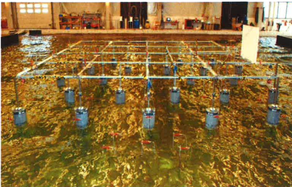
Fig. 1. The 25-WEC farm in the DHI Shallow Water Wave Basin (Hørsholm, Denmark) under irregular long-crested waves. View from behind the wave generator. Top: aligned ; bottom: staggered lay-out.
