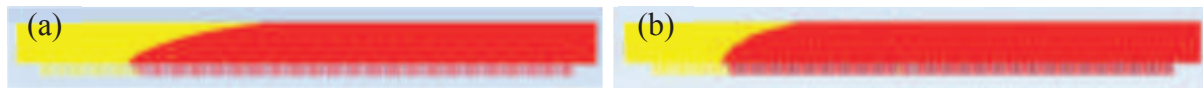
Figure 4: Refreshment state of irradiated LBE (yellow) in (a) concept 1 and (b) concept 2 100 ms after arrival of a proton pulse. Red color represents non-irradiated LBE.
