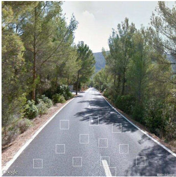
Fig. 6. Extraction of sub-images from the road surface. We extract 32 \times 32 pixel sub-images of different road surfaces to form the road image dataset.
