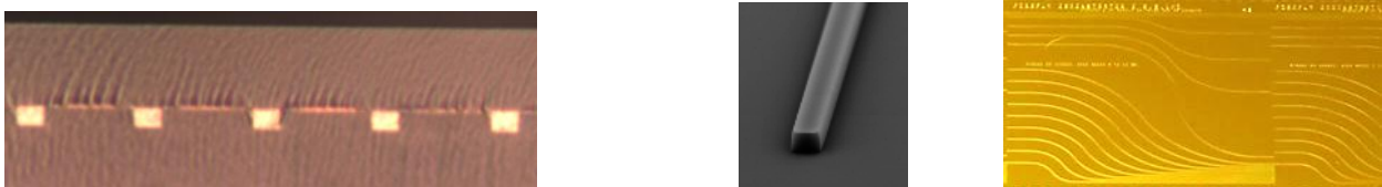
Figure 2. Imprint-based OrmoCer waveguides: left) Cross-section of five parallel inverted-rib waveguides, showing very thin (0.5 \mu\text{m} ) slab layer; middle) SEM of ridge waveguide with end facet; right) Waveguides of varying bend radii on a wafer.
