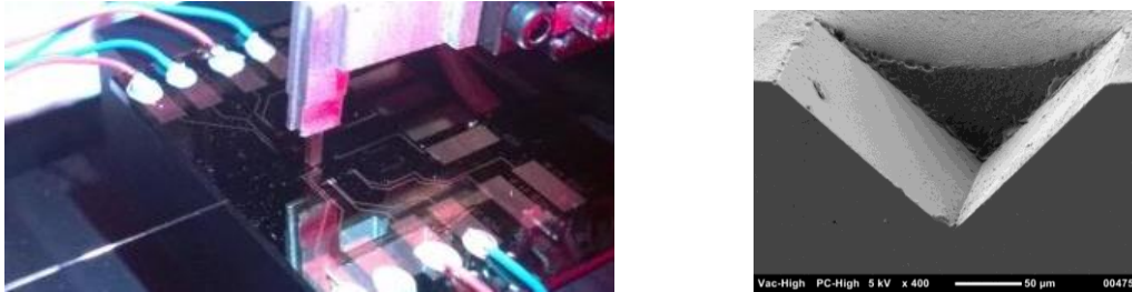
Figure 10. Coupling mirror imprinting: Left) Sample chip with waveguides and embedded VCSELs under the mirror imprinting mold in the precision alignment station. Also the monitoring fiber used in the active alignment is seen. Right) SEM image of a mirror imprinted in OrmoClad by the micro-prism mold. (Note: the residual particles are from the dicing, which was used to make the cross-section sample for SEM.)
