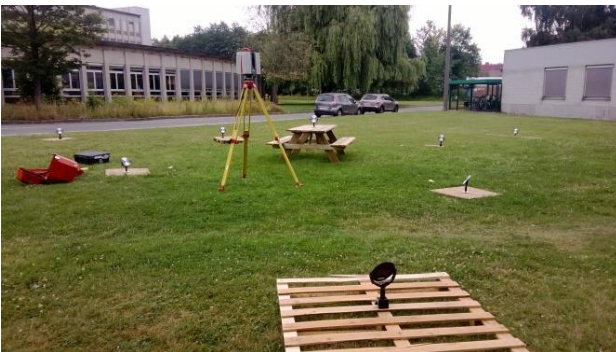
Figure 4. Configuration of laser scanner and targets
