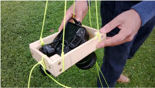
Figure 3. Wooden frame supporting camera
