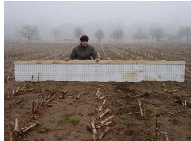
measuring surface roughness with 4-m meshboard
