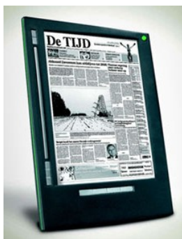
Figure 1: The newspaper 'De Tijd' experiments with a display from I-Rex based on electrophoretic ink, a technology developed by Philips and E-Ink.
