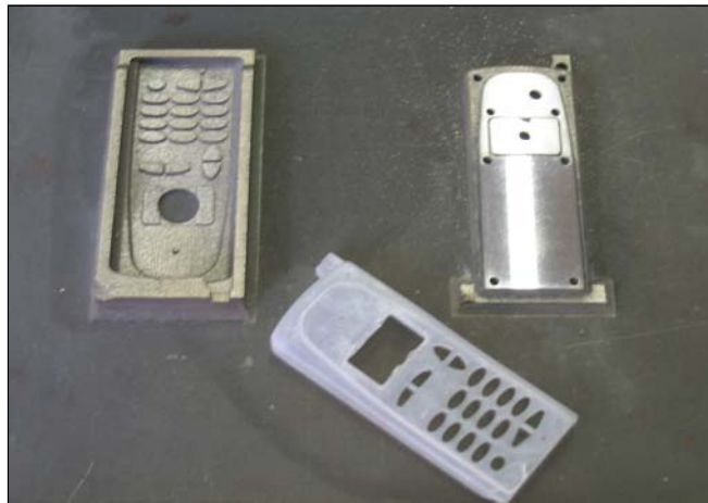
Fig. 2. The difference between an unpolished and polished SLS mould surface. Cavity half is unpolished; core is polished. Moulded part also shown (under).
