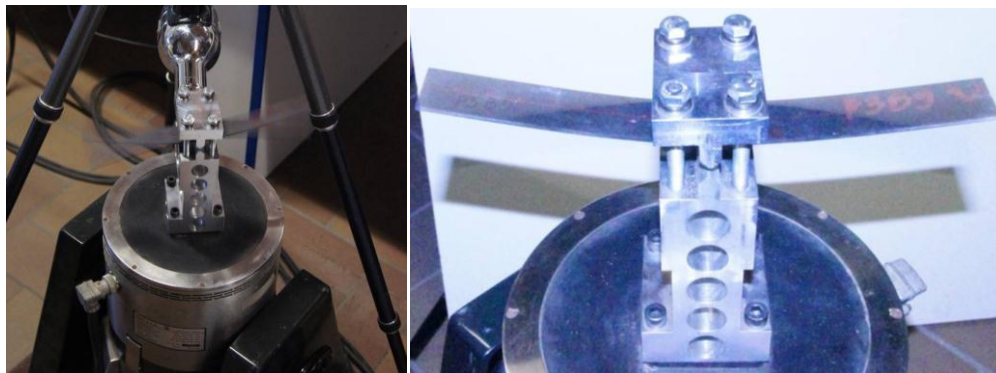
Figure 1 – Accelerated fatigue testing with an electro-magnetic shaker
