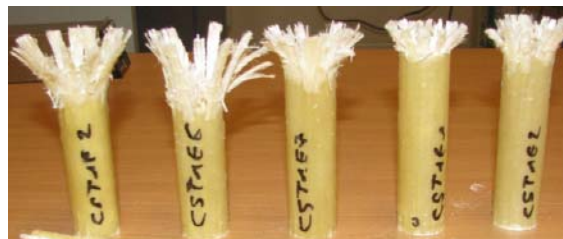
Figure 2. Uniform progressive crushing of the circular cross sectional glass polyester composite tubes (1 mm wall thickness) for different charge mass and stand-off distances (20g and 30g with 30 cm stand-off distance).
