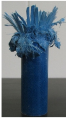
(a) Deformation pattern of commercially available pultruded GFRP composite tube (2 mm wall thickness) with triggering type 2 for 40g of C4 with 15 cm stand-off distance.
