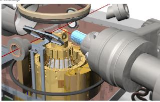
To minimize interfering mechanical stress on the sample holder, especially during movements, it is mechanically decoupled from the cold reservoir. The sample holder is cooled by a circular array of highly flexible Cu wires between the sample stage and an outer cold cylinder that moves in synchrony with the sample rotation stage in order to keep the strings slack. The cooling cylinder itself is cooled by spring loaded sliding connectors attached to the cold reservoir.
