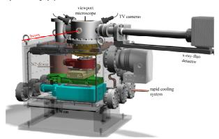
The cryogenic environment consists of a two compartment vacuum system, two cooling systems, an X-ray fluorescence detector with ultrathin polymer window for e.g. fluorescence tomography, a PCO camera for full field absorption and phase contrast tomography, sample stages as well as components like a zoom-microscope for visual light observation (co-linear with the beam and top view), and TV cameras. A shuttle system for cryogenic sample loading in vacuum is currently being added.
