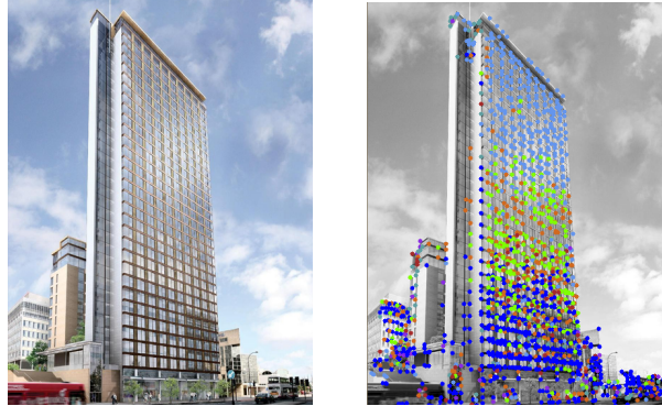
Fig. 10. Corner detection, the color gives a coarse indication of the corner angle.
