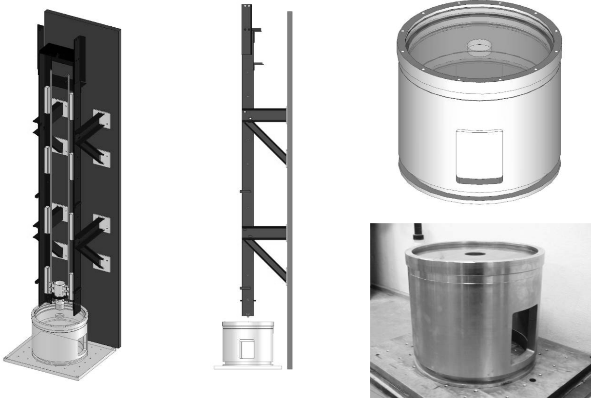
Fig. 1. Drop weight set-up for impact on circular glass specimens.
