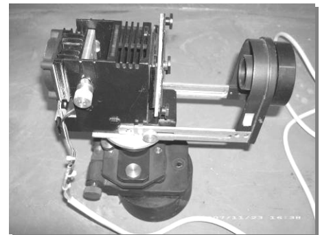
Fig.4. Fringe projection device. Schematic presentation (a), picture of the device (b).
