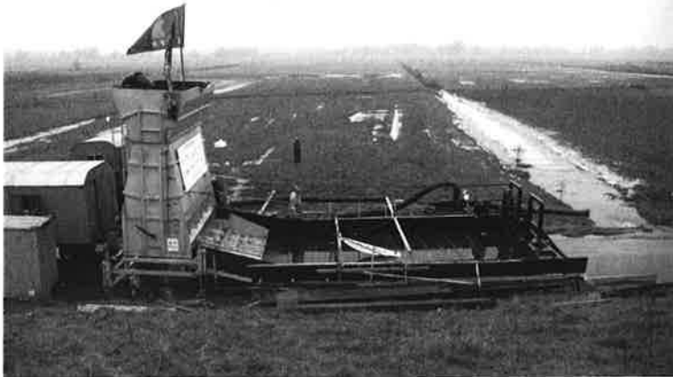
Figure 9 Set up of the overtopping Simulator and storm return walls
