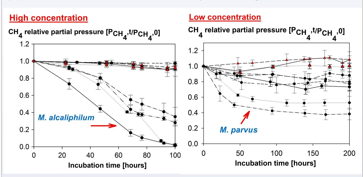
Among all building materials, **Maastricht limestone** (graphs above) provided the best support for the highest methane removal by MOB at high (99.9% removal after 100 hours by M. alcaliphilum) and low concentration (64% removal after 200 hours by M. parvus)
