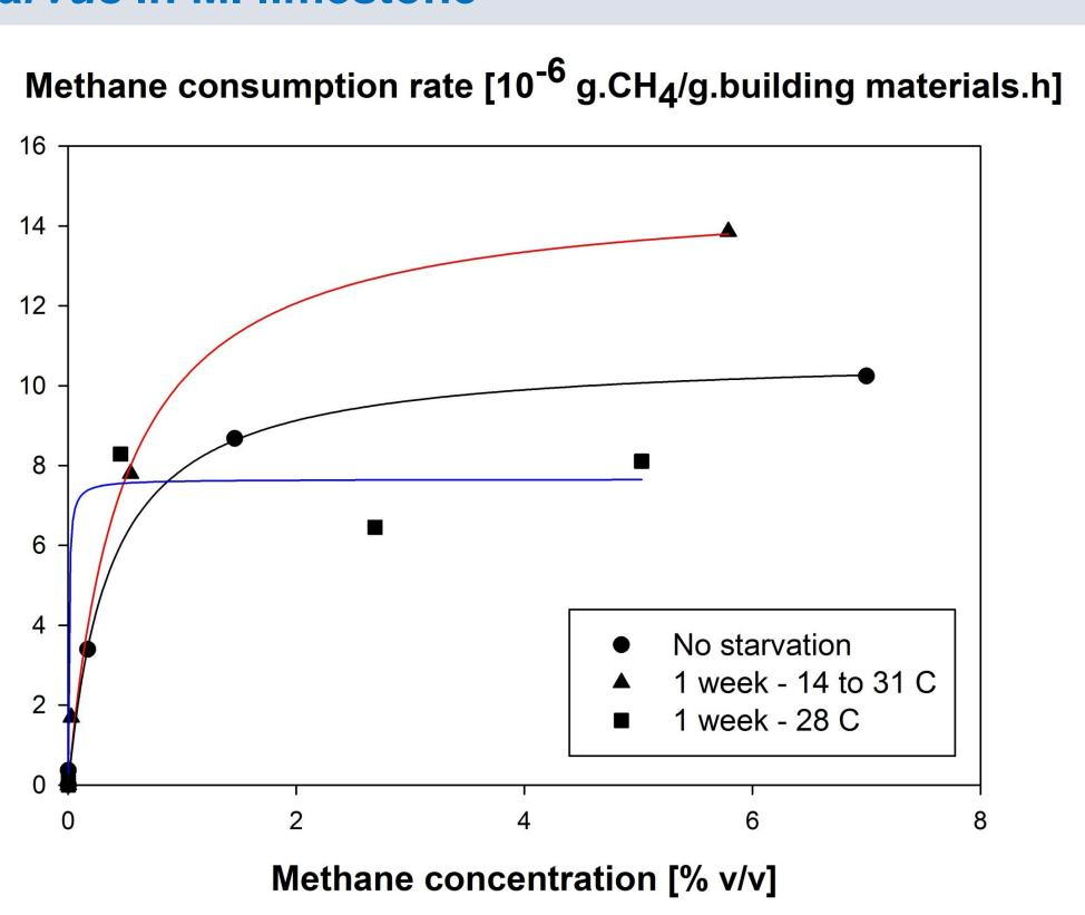
Bacteria could still remove methane after 1 week of methane deprivation at varying or constant temperature with altered methane removal kinetics
