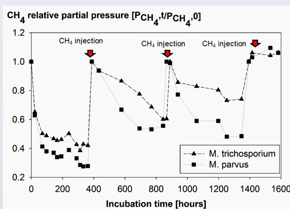
With pulse feed methane injection process, MOB could still remove methane at low concentration for approximately **2 months**
