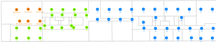
Figure 1. Third floor of the w-iLab.t testbed at the IBCN buildings. Floor area is approximately 90m x 18m.
