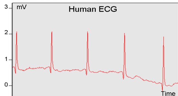
Fig. 8. Top: the finished ECG-sensor device. Bottom: the measured ECG signal at the receiver side.
