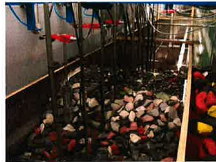
Figure 6 : Wave gauges in perforated tubes (stage 2)
