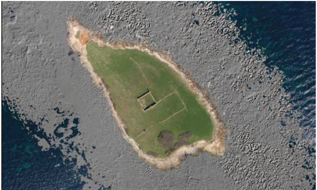
Fig. 5: Palacol. Combination of orthophotograph and ALB-derived DTM. The DTM is shaded with a light source in NW.
