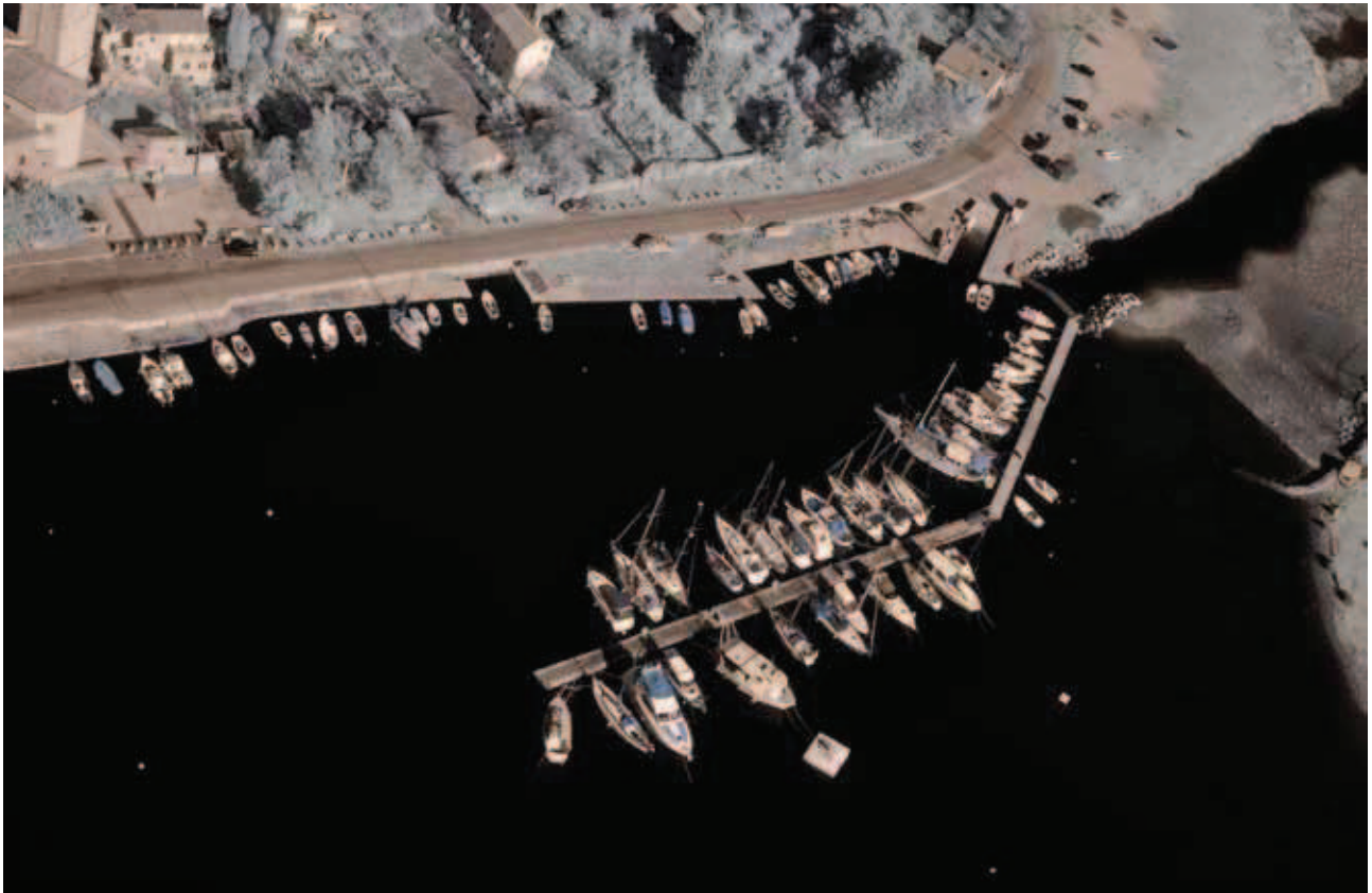
Fig. 1: Near-Infrared aerial photograph of the harbour in Osor. Because electromagnetic Near-Infrared wavelengths are almost completely absorbed by water, the sea is rendered black.
