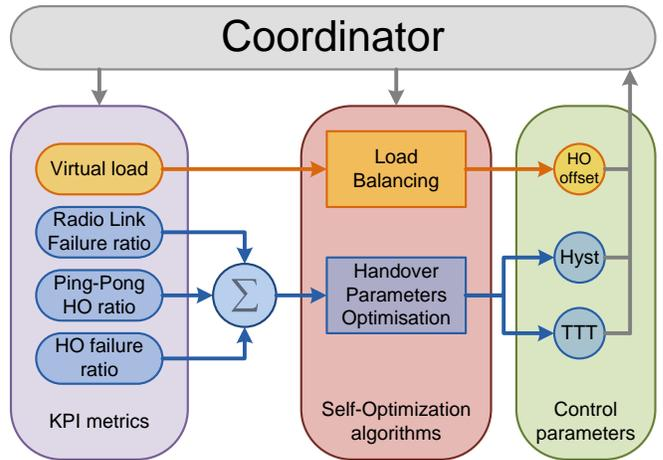
Fig. 6. Coordinator scheme for HPO and LB algorithms
