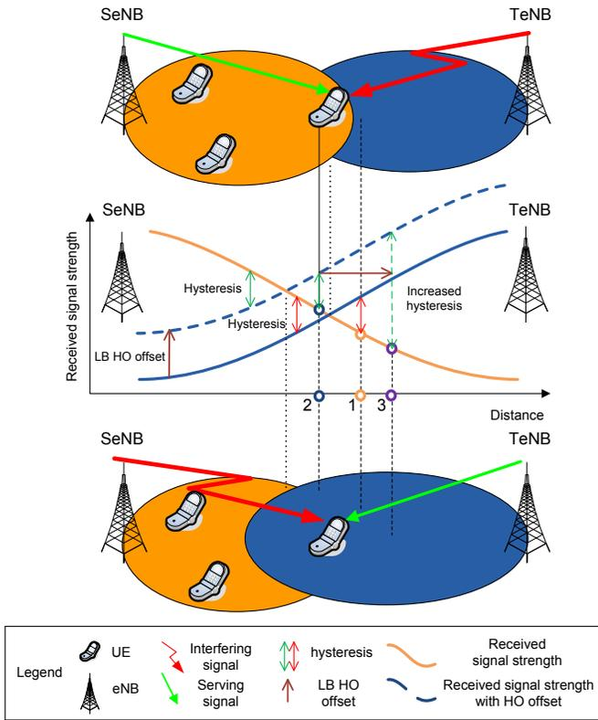
Fig. 3. Load Balancing and Handover Parameters Optimisation interaction
