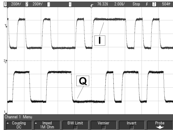
Figure 6: I-signal and Q-signal as function of the time.
