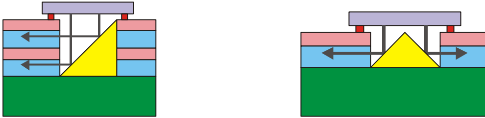
Figure 3: Schematically representation of the use of deflecting structures to couple light from VCSEL-arrays into (stacks of) waveguides. This also clearly demonstrates the possibility to fully exploit the 2-dimensional character of the arrays.
