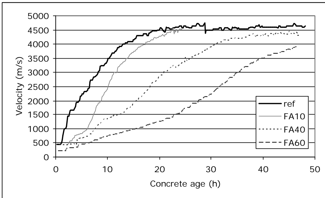
Fig. 4. Ultrasound pulse velocity for concrete types with different fly ash content
