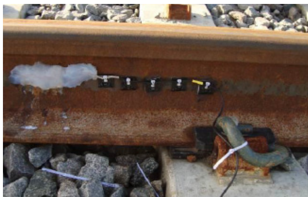
Figure 5: Strain gauge on a rail track.
