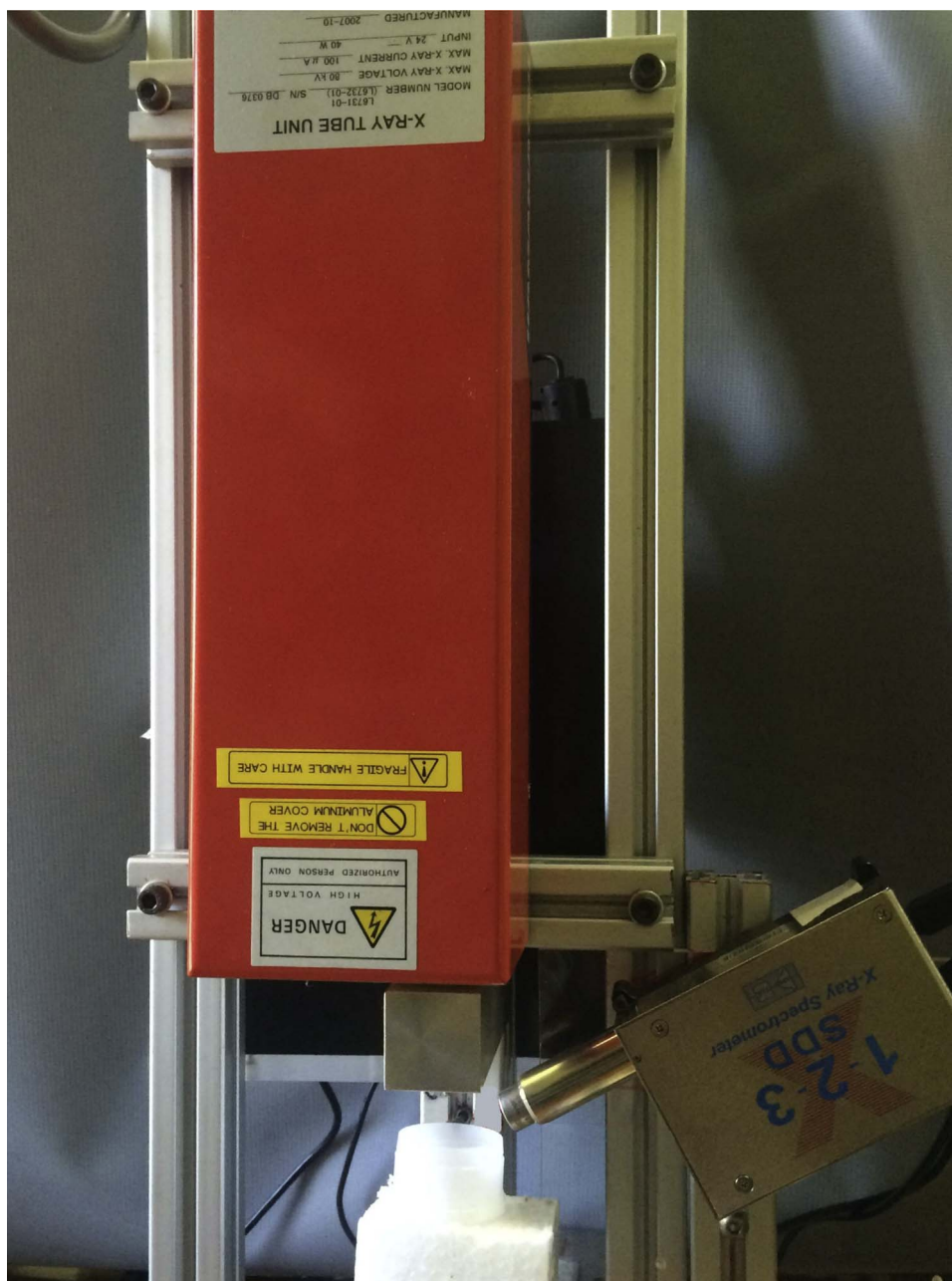
Fig. 1. Image of the X-ray fluorescence setup utilized in the analyses.
