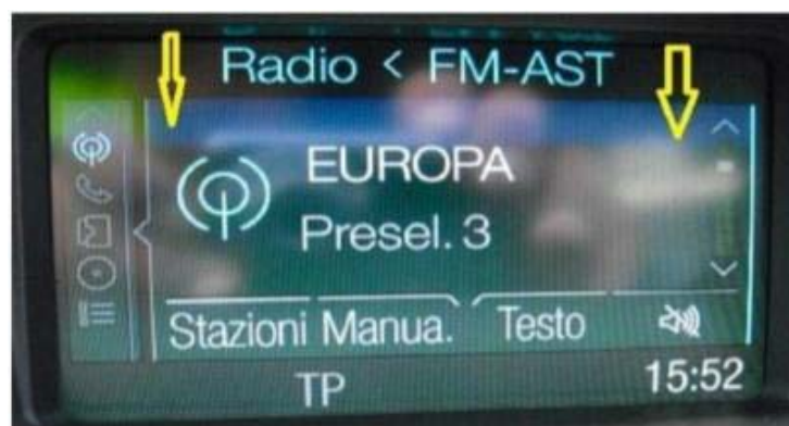
Figure 2 – Example of display contamination
