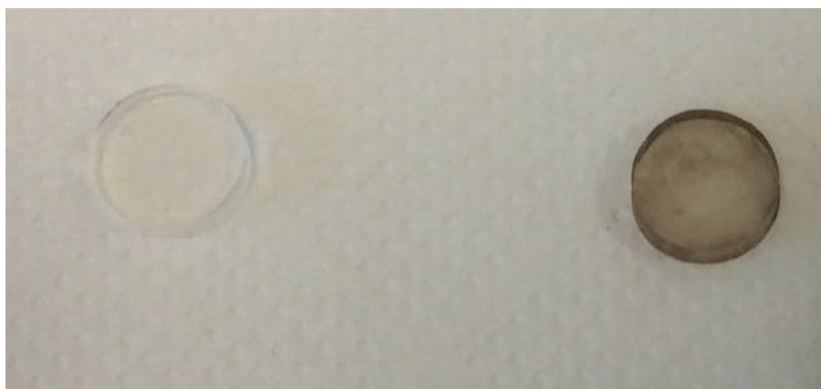
Figure S1. Polydimethylsiloxane samples before and after pDA deposition.
