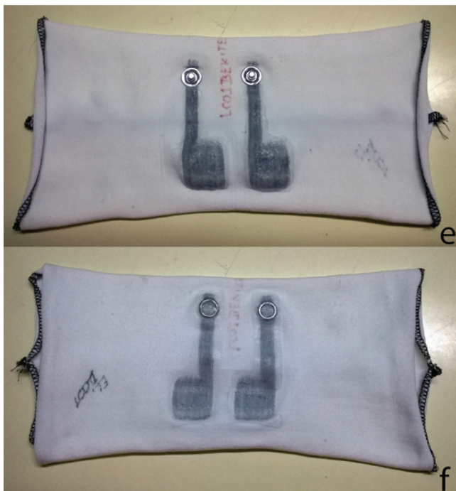
Figure 3. LC01 Electrodes knitted in a sleeve with silicone as the impermeable membrane: e) front; f) back
