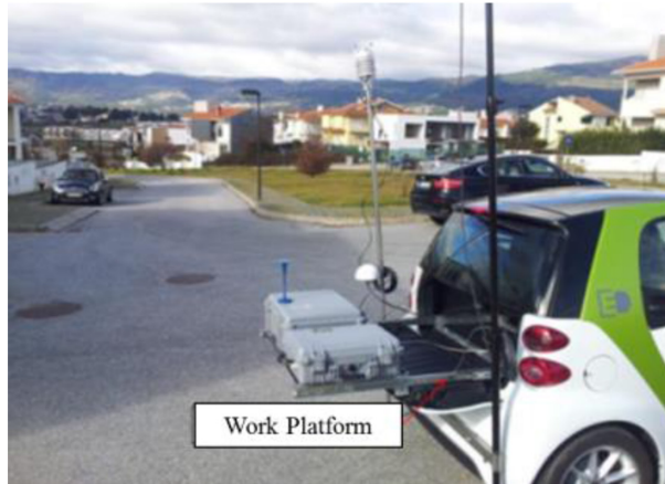
Figure 2: Sliding work platform.
