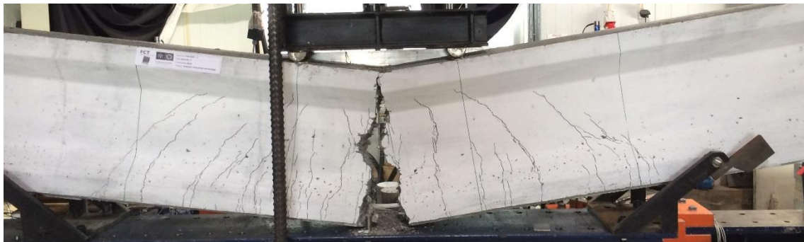
Figure 5-48: Failure of specimen IB9 after about 1.82 Million of fatigue cycles
