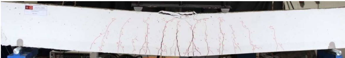
Figure 6.14: Propagated damages at the end of the test of FB_R
