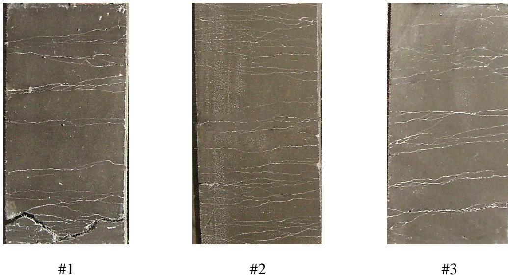
Figure 4.19: Diffused multiple cracking in the gauge length of the un-notched specimens prepared with composite mixture C4W30 and subjected to the tensile loading
