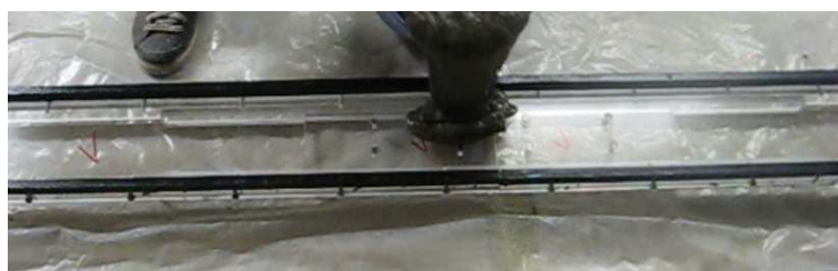
Figure 6.6: Casting of the SHCC plates from the mid-length of the acrylic molds
