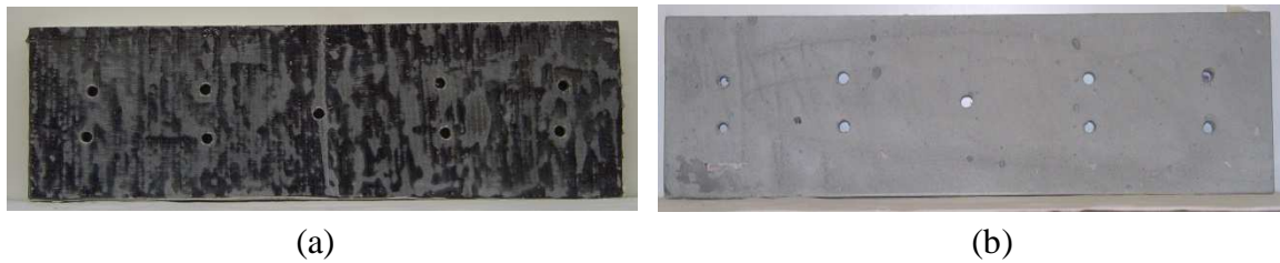
Figure 4.31: Perforated HCP (S) , (a) the face with bonded CFRP sheet, and (b) exposed face
