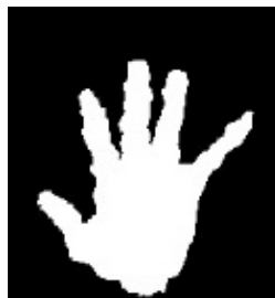
Figure 14. Hand blob extracted from the depth image and used for feature extraction.
