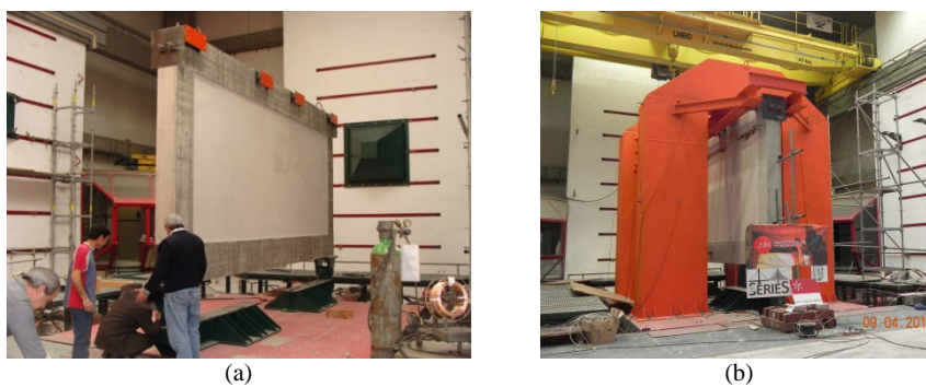
Fig. 16.20 Wall panels test setup: (a) Hinged base and pyramidal support; (b) complete setup.
