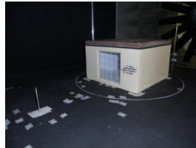
Fig. 7. Model positioned inside the tunnel.
