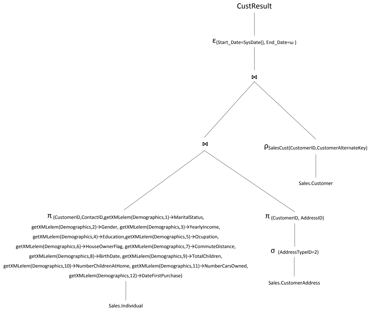
Figure 29 – RA tree with the representation of the RA expression presented in Section 3.4.1
