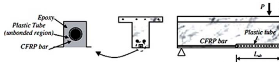
Figure 2-4: Configuration of partially bonded beams (Choi et al. 2011a)
