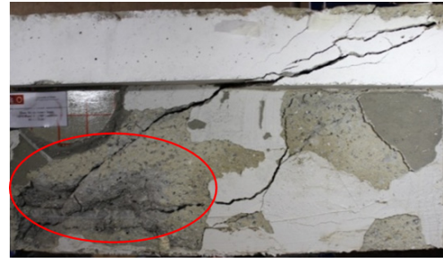
(b) Final crack pattern of the SP-3L45-II beam when HCP was peeled off after the test
