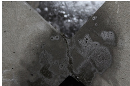
Figure 5-11: Typical crack patterns Iosipescu specimens tested
