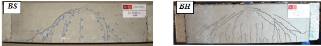
Figure 2-31: Typical cracks pattern and the failure modes of the beams (Esmaeeli et al. 2013a)
