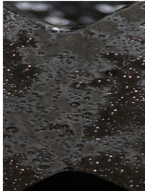
(b) Crack pattern at second phase (nonlinear pre-peak)
