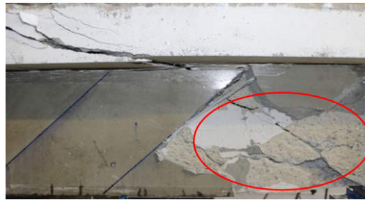
(c) Local detachment of HCPs at failure load
