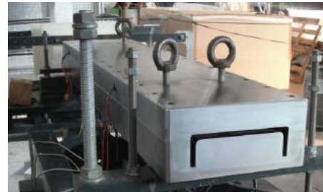
a) Die mounted on the pultrusion equipment
