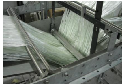
Fig. 3. guiding mechanism used at the resin impregnation basin
