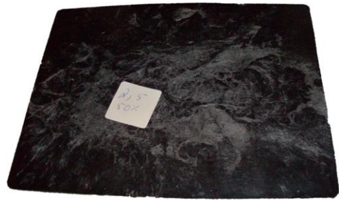
Fig. 9. Final stamped GF/PP LFT composite plate
