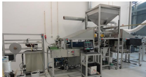
Fig. 5. Prototype coating line used to produce towpregs
