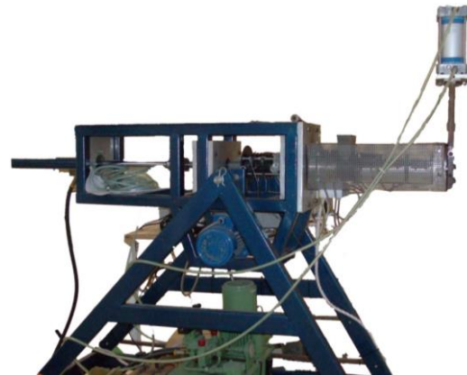
Fig. 7. Photograph of the piston-blender used in the present work
