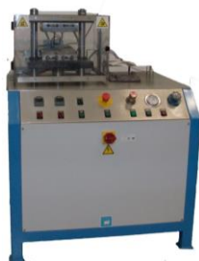
Fig. 8. Hydraulic press used to stamp the final GF/PP LFT plates
