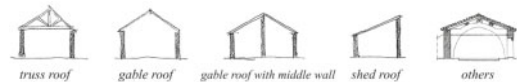
Figure 19. Types of roofing systems usually observed in this building typology (credits: J. Ortega).
