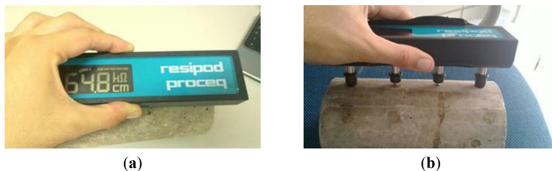
Figure 4. Visualization and measurement of the electrical resistivity. (a) electrical resistivity apparatus; (b) measuring electrical resistivity.
