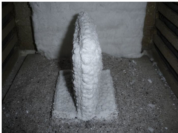
Fig. 2: Example of T steel structure inside the furnace after a thermal insulation test. Notice the white intumescent foam that remained on the structure
